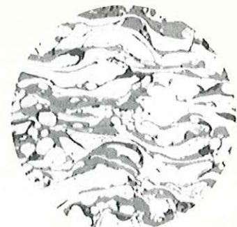
Spraying material : SUS 410 (13% Cr stainless steel)(200 magnifications)
